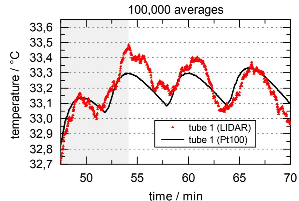
✓ Average Deviation  $0.07^\circ\text{C}$  ( $\triangleq 810\text{ kHz}$ )
